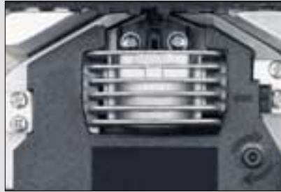
Printing unit: simple ribbon replacement
